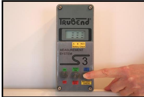
Flip and hold the battery check switch to check the battery condition.
